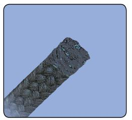
Diagonally braided from high-quality textured glass fibre, impregnated yarn by yarn with pure graphite powder and a corrosion inhibitor.
